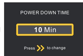
**3.5.1** The power down time is adjusted according to “>” and the power down time increases from 3 to 20 minutes (3-5-10-15-20), which is the so-called stop time of the fan after shutdown, in order to better drain the water. Factory set for 3 minutes.(the other state of the fan is still 15 seconds.)
