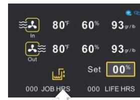
**"Pump working countdown"**: indicates: No matter in which working state and interface, as long as the pump works, this interface appears and counts down to 28 seconds. However, the interface only displays the previous working status and interface after 3 seconds. For example, after 3 seconds, there is a drainage icon on the main interface and it will flash until the drainage is finished.
