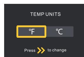
**3.6 Temp Units °F/°C**: Used for temperature scale switching. Press the “>” button to switch °F / °C, after switch symbol of corresponding parts is also changing.
