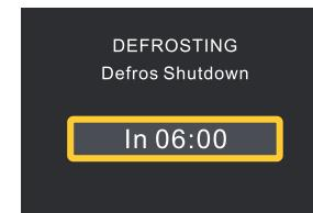
When the machine is running normally, “Defrost SHUTDOWN IN 06:00” will occur in the interface after defrosting. It’s defrost countdown use seconds as units. This screen displays only 3 seconds. Displays the previous interface and status after restoration. If it is the home screen, the frost icon will flash.
