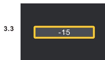
**3.3 Coil Temp 000°C**: Used to display the current temperature of the coil. When it is below zero, the “-” symbol is displayed in front. “-” is not required on zero.
