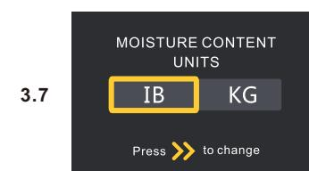
**3.7 MOISTURE CONTENT UNITS**: It is used to switch the unit of GPP value with moisture content. Press > to switch the lb or Kg, after switch symbol of corresponding parts is also changing.
