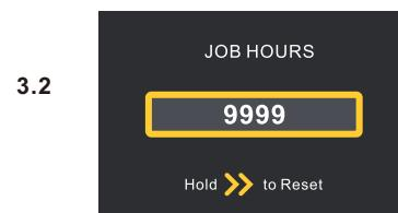
**“Indicates”:** Do I need to clear out this time? “>” if you need to clear. When the operation is completed, the working time of the main interface and the working time of this interface will be reset and started to be instant again. After accumulation (9999), clean up and round.
