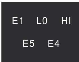
Make fault judgment and take corresponding actions after starting up. Regardless of the state, the fault is executed first and the fault code is displayed on the interface. If there is a fault in the sub-menu operation, immediately return to this interface display fault (including defrosting state). (the fault is judged when the pump works, and the fault is displayed as usual, but the pump needs to complete the water pumping this time). Multiple faults can be displayed at the same time.
